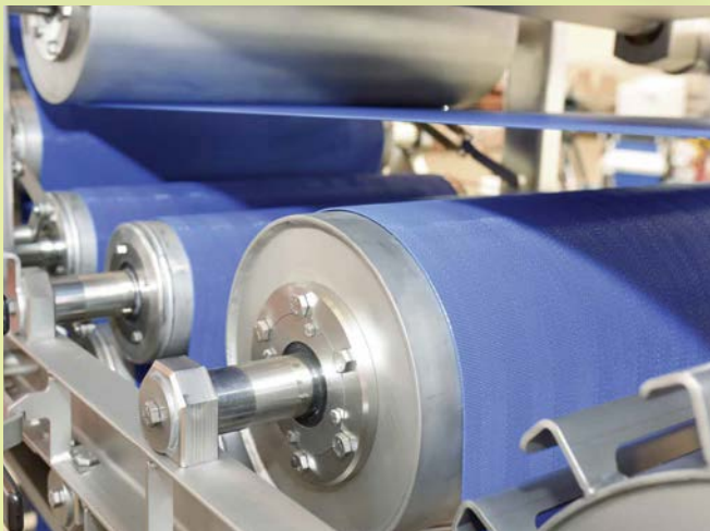
The total of twelve press rollers in the high pressure zone are arranged on a single level resulting in an overlap-free arc of contact, which optimises yield.
