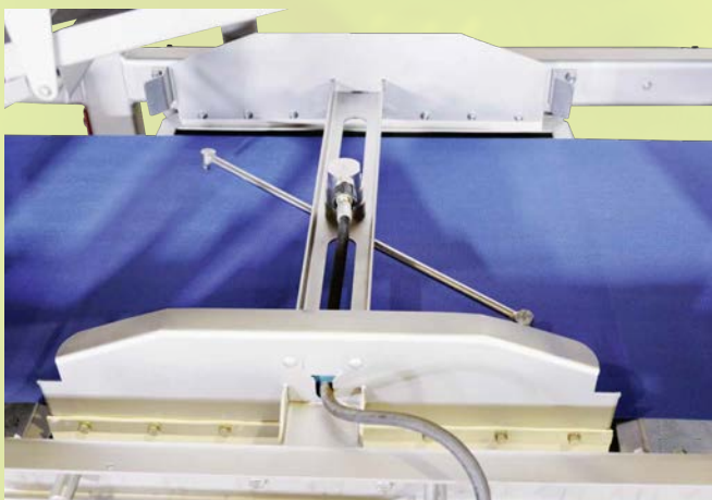
Both belts are cleaned by a high-pressure-cleaner during operating.
