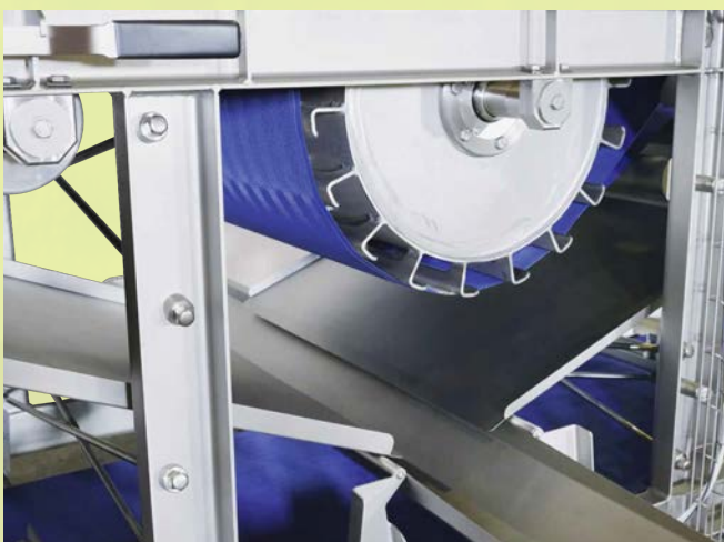
The special open construction of the main press roller guarantees fast and unhindered penetration and drain-off.
