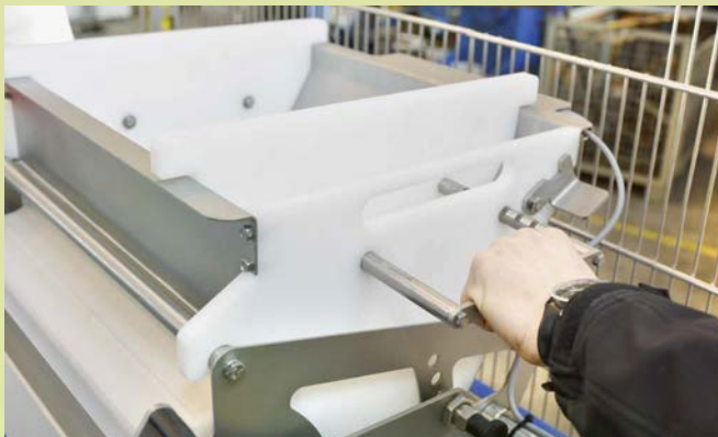
Adjustable feeding hopper for different mash-width'
