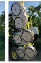
The orientation of the heads increases or decreases the removal intensity. A multitude of possible combinations to adjust your working height.
