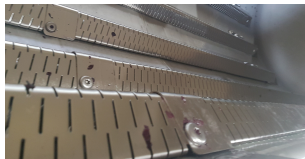
Electropolished draining channels, quick-fit without tools
