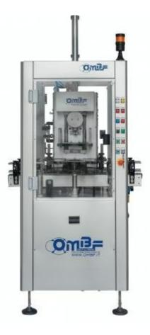
The automatic Wire-hooder, MINI version, 2015A-2TR/10 model is the new entry of the OMBF's range of automatic wire-hooders. With its hourly throughput of 1500 bottles, it is the smallest of the range, designed to the inserted in low production bottling lines.
