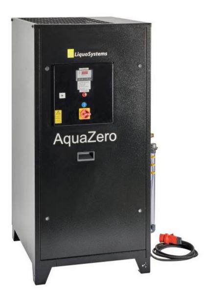
The Chiller is compact and easily connectet to an existing pipeline system. They are equipped with a water tank and centrifugal pump. In outlet temperatures below + 10 ° C is the use of antifreeze (glycol, 34%) required.
