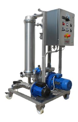
Crossflow filtration makes a perfectly clear product without any clarifying agent and/or filter aid requirement. When a clarifying treatment with bentonite or other clarifying agents is required, it is necessary to wait for the decantation and transfer the clear product in another tank before starting filtration. Filtration rates and cycles of filtration are depending of solid's content and kind of products such as colloids, bacteria, yeasts.
