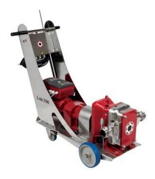
The Delta LOB pump has food-certified hard nitrile lobes. It allows solid particles up to 25 mm in diameter to pass through. Self-priming, this pump can run dry up to 8 metres. It offers the utmost respect for the wine, with a continuous flow without stirring. It is highly resistant to temperature (from -10°C to 90°C) and pressure (from 4 to 10 bars depending on the model). This lobe pump dissolves very little oxygen and allows solids to pass through.
