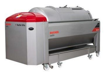
The Bucher XPro is designed to process whole bunches, destemmed and / or crushed grapes as well as fermented pomace. This grape press is especially dedicated for a selection of qualitative batches. Very easy to handle and to use, very compact, the Bucher XPro press fits easily in every winery.
