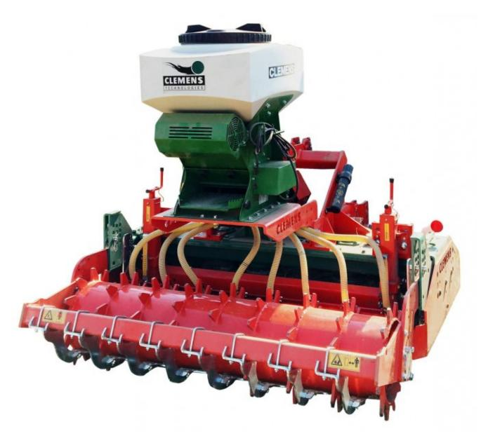
The pneumatic seed drill offers many advantages. The electrically controlled seed shaft transports the seed from the container into the air channel. Here the seed is conveyed with the aid of the blower via flexible hoses to the baffle plates and distributed evenly and close to the ground. This ensures exact seed application even in windy conditions!
