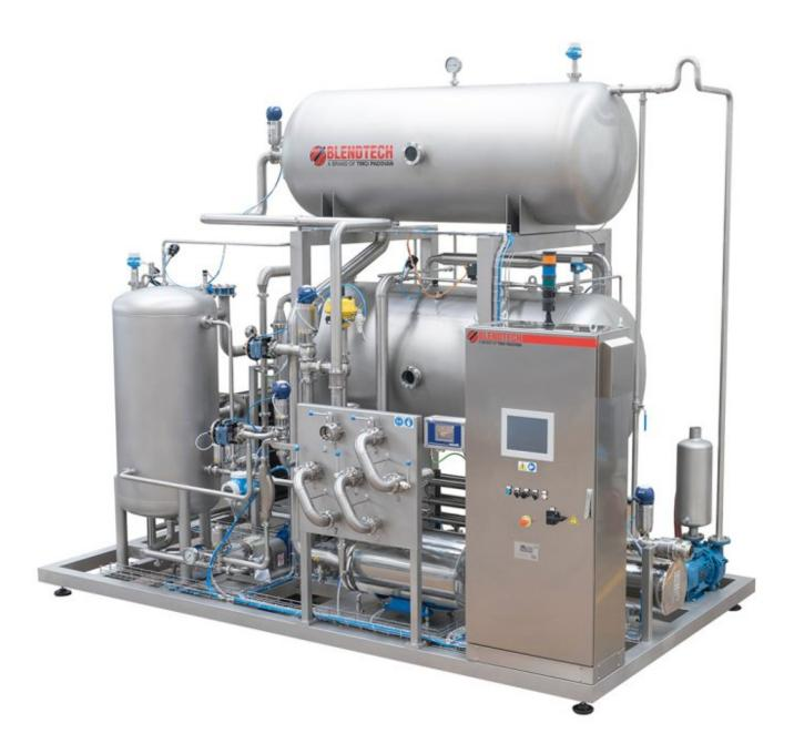
The BLENDTECH Premix monoblock device is a complete system for the preparation of carbonated soft drinks by mixing the syrup with deaerated water and then carbonating it. Two or more ingredients are mixed together in different proportions set by the operator, depending on the type of end result required.
