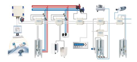
The VinInfo is a modular system in every aspect. The building-blocks of the VinInfo management system are the BU - the 'Basic Unit'. Each tank and each additional item (pumps, room acclimatization units etc.) is regulated by its own BU. All BU in the cellar are connected with a single BUS cable running between them and then to the Server-PC. More BU's for control of additional equipment can be added at any time, at any place along the cable line – cut (the cable) and connect (another BU).
